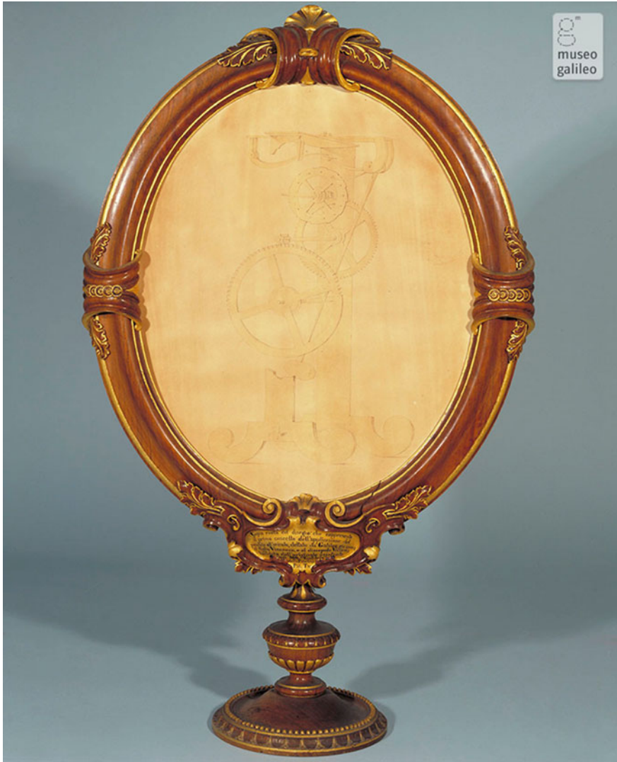
Fig. 7 Copy of the design of Galilei's clock mechanism by Vincenzo Viviani and Vincenzo Galilei. Copyright of Museo Galileo , photographic archives, Florence
