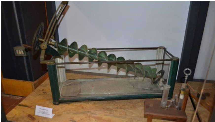
Fig. 19 The model by Prof. Francesco Masi (1890) (Ceredi 1567 ), recently discovered and displayed at the Museo del Patrimonio Industriale in Bologna. The static seal between the screw and the external prismatic tube realized with 12 strips of glass was made using a leather square wire. This model was displayed and awarded in Paris at the Universal Exhibition in 1867 (Ceccarelli 2005 )
