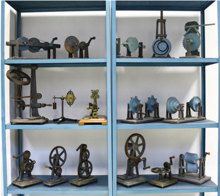
Fig. 3 Didactic models of elementary and complex mechanisms used in TTM lessons at the University of Palermo at the beginning of the 19th century, (Monastero and Genchi 2012). Courtesy of the Museum of Engines and Mechanisms
