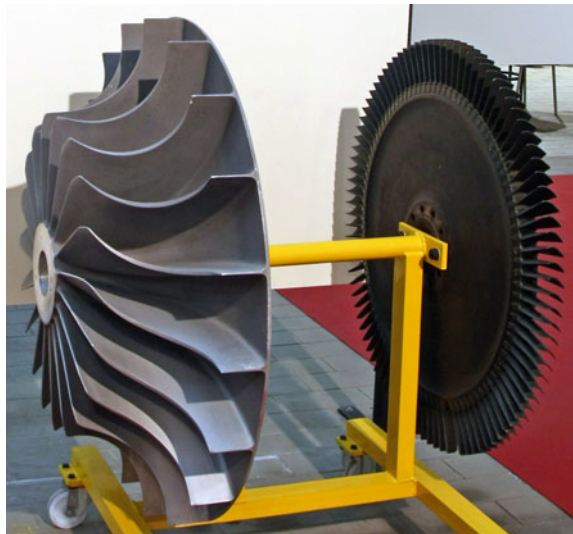
Fig. 18 Turbojet engine de Havilland Ghost: compressor and turbine impellers
