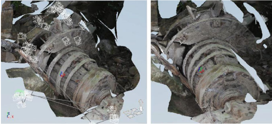
Fig. 16 Photogrammetric three-dimensional reconstruction of the vertical wheel and camshaft for copper processing in Villa Tordinia mill. The reconstruction was realized with the software Autodesk 123D Catch
